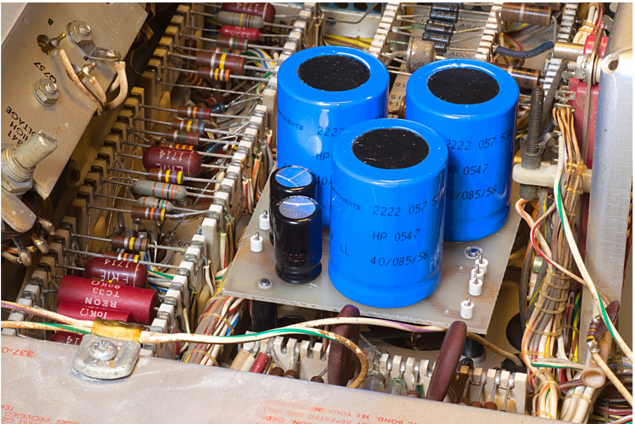
Image 1: First PCB with main filter capacitors (not connected yet)
