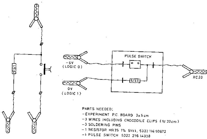
Before switching on the tests, connect the test switch to the PM2528.
