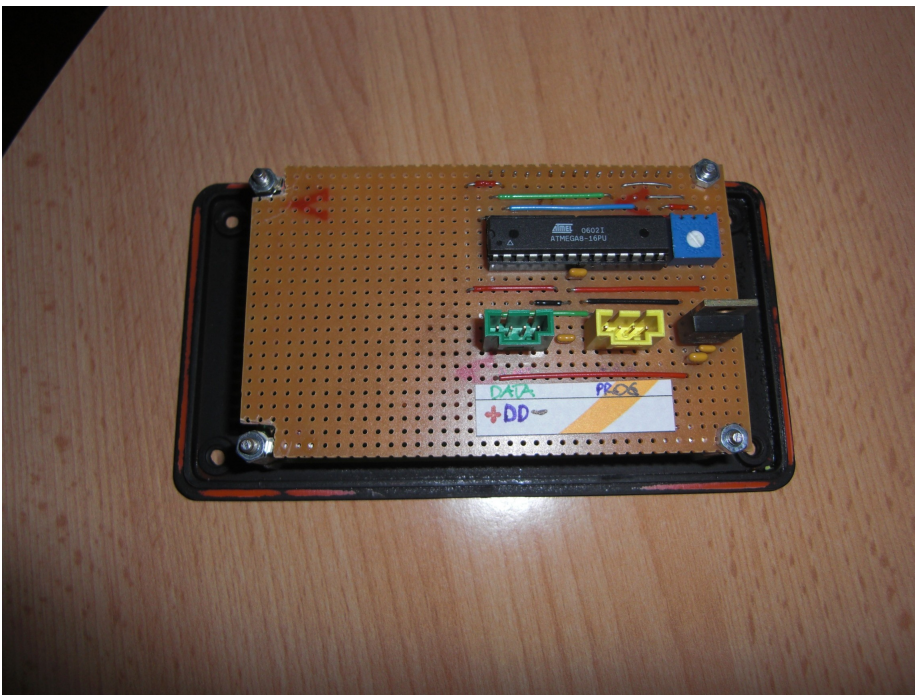
Picture 5: The too-simply circuit may even be constructed using prototype-PCBs.
