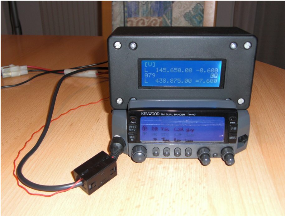
Picture 4: The external display for the TM-V7 ready for action!
